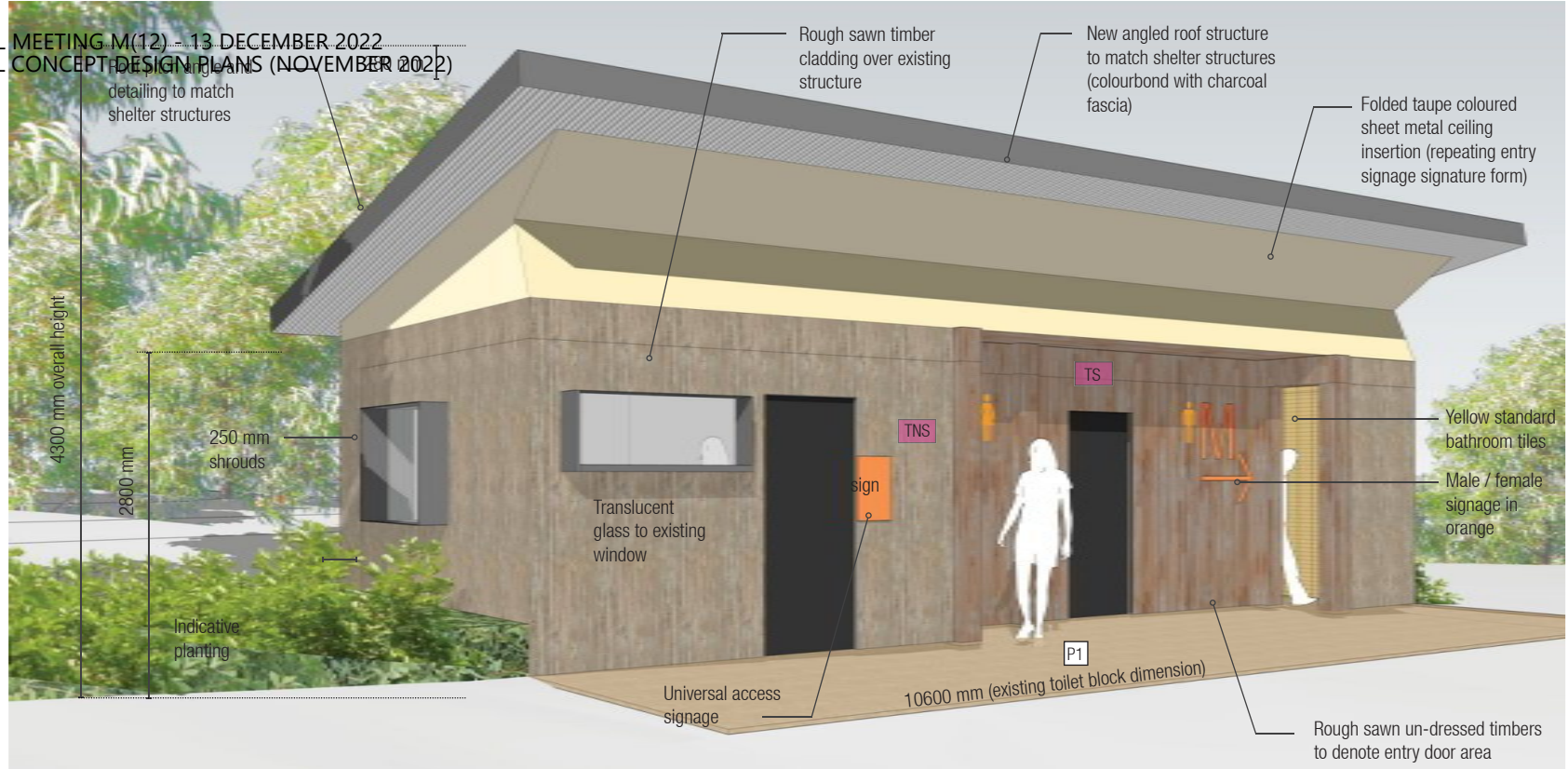
Toilet retrofit view 1
