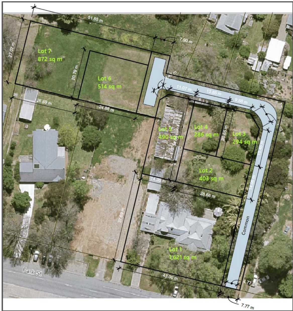
Figure 1: Shows the development layout on site.
