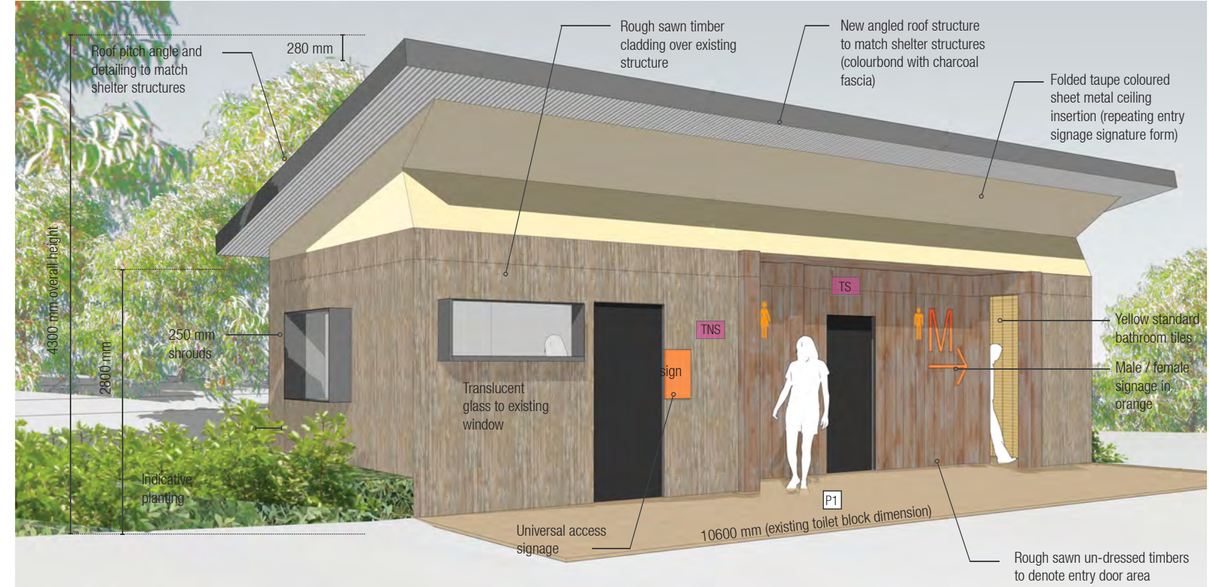
Toilet retrofit view 1
