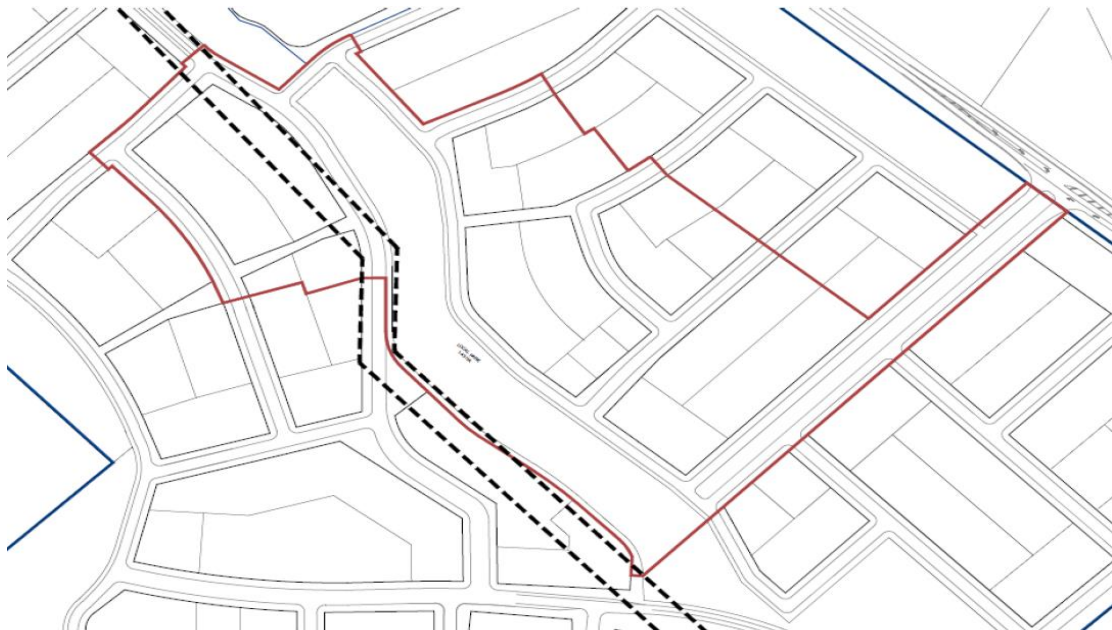
Figure 8: Existing road reserve and proposed road network
